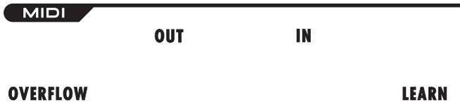
The MIDI **OUT** connection functions as a thru as well. The MIDI **IN** is self-explanatory. The **OVERFLOW** switch sets the MIDI overflow parameters for chaining multiple Boomstar synths together. To do this, activate the first unit's **OVERFLOW** switch, and the last unit in the "chain" **OVERFLOW** switch disengaged. Note: For proper
